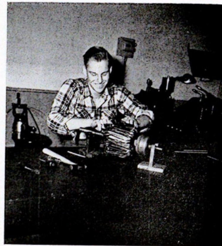
Rewinding an armature is an important part of the electrical student's training. Here the job is getting the full attention of Gordon Olson of Forman.
